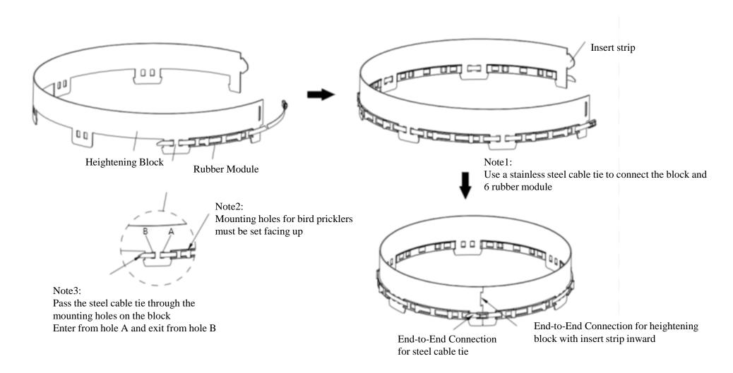
Step3: Tie the Heightening Block on Rain Cylinder Funnel
