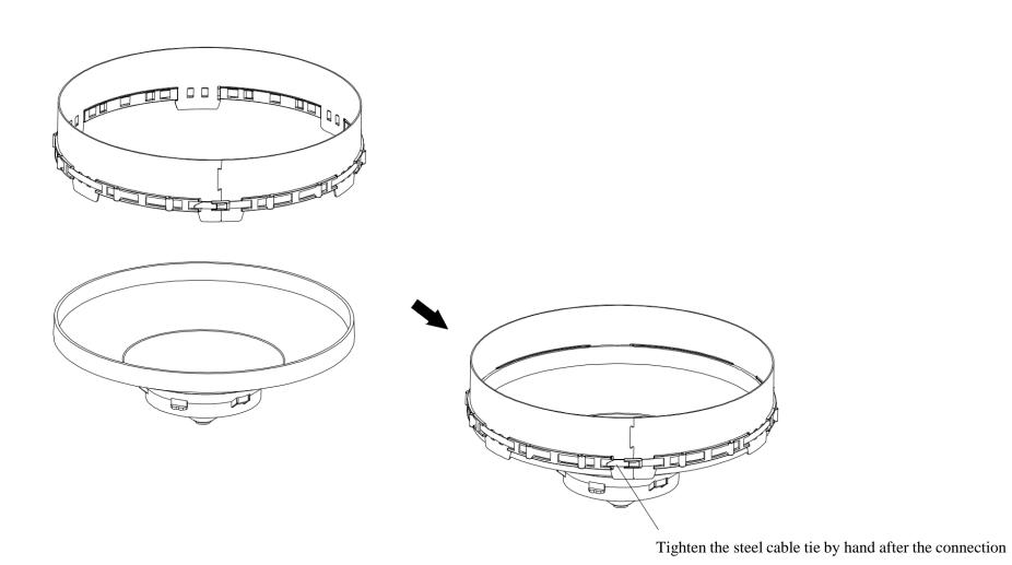
Step4: Tighten the Steel Cable Tie with Needle Nose Pliers
